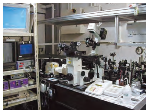
Fluorescence microscope system for imaging single molecules within living cells
